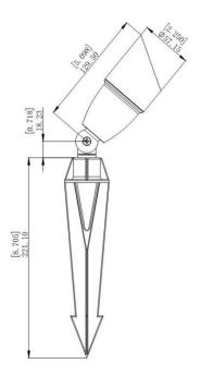
Material: Brass Voltage: 12VAC Bulb Type: MR16 Maximum Wattage: 35W IP Rating: IP54 Wire:SPT-2W/18AWGX2C
